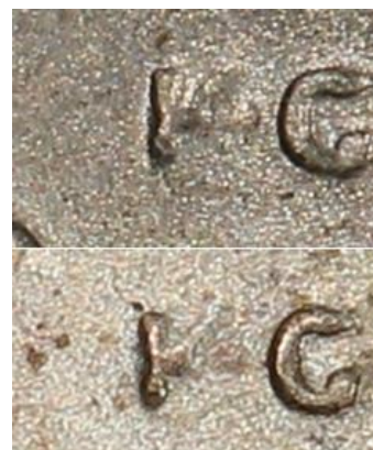
Fig 15. Damage to K of KG (designer’s initials) on 1946 Melbourne (top) and Perth (bottom) shillings due to damage to transfer punch used in manufacturing all dies used at both mints. Photographs courtesy of PCGS.
