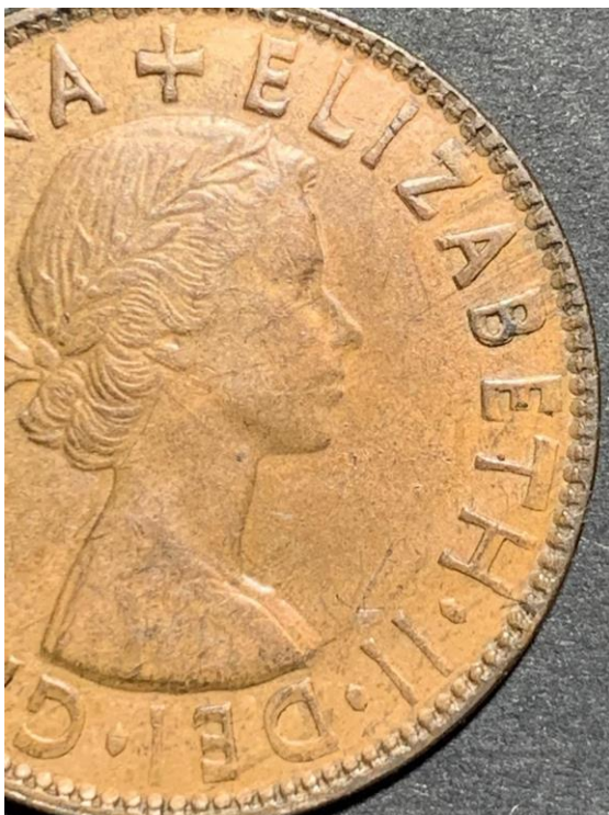
Fig 5. Mishubbing, spreading of the die during die manufacture on a 1954Y halfpenny. It is unclear whether this occurred on the first or second press of the transfer punch.
