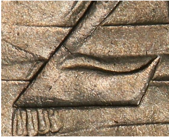
Fig 10. Wavy 2 twenty cent, caused by damage to the die before it was used to strike coins. Photograph courtesy of PCGS.
