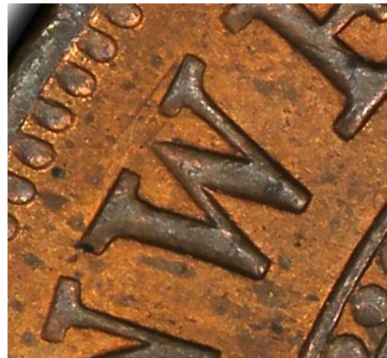
Fig 20. Closeup of W in COMMONWEALTH on 1920 double dot penny. The two lines above the W were caused by damage to the working die before any coins were struck. All 1920 double dot pennies have these lines. As the bottom dot is subject to die fill, this characteristic is useful in determining whether a coin is a double dot or a dot above top scroll. Photograph courtesy of PCGS.
