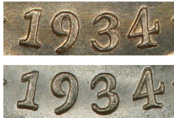
Fig 13. 1934 sixpence date varieties. Narrow date (top), wide date (bottom). These arise from dies derived from different 1934 dated master dies. Notice how both the 3 and 4 are in different positions, suggesting that the partially dated master die was dated 19. This is not surprising as no sixpences had been produced since 1928 and the Melbourne Mint would have derived both dated masters from a 192 dated master die. Photographs courtesy of PCGS.
