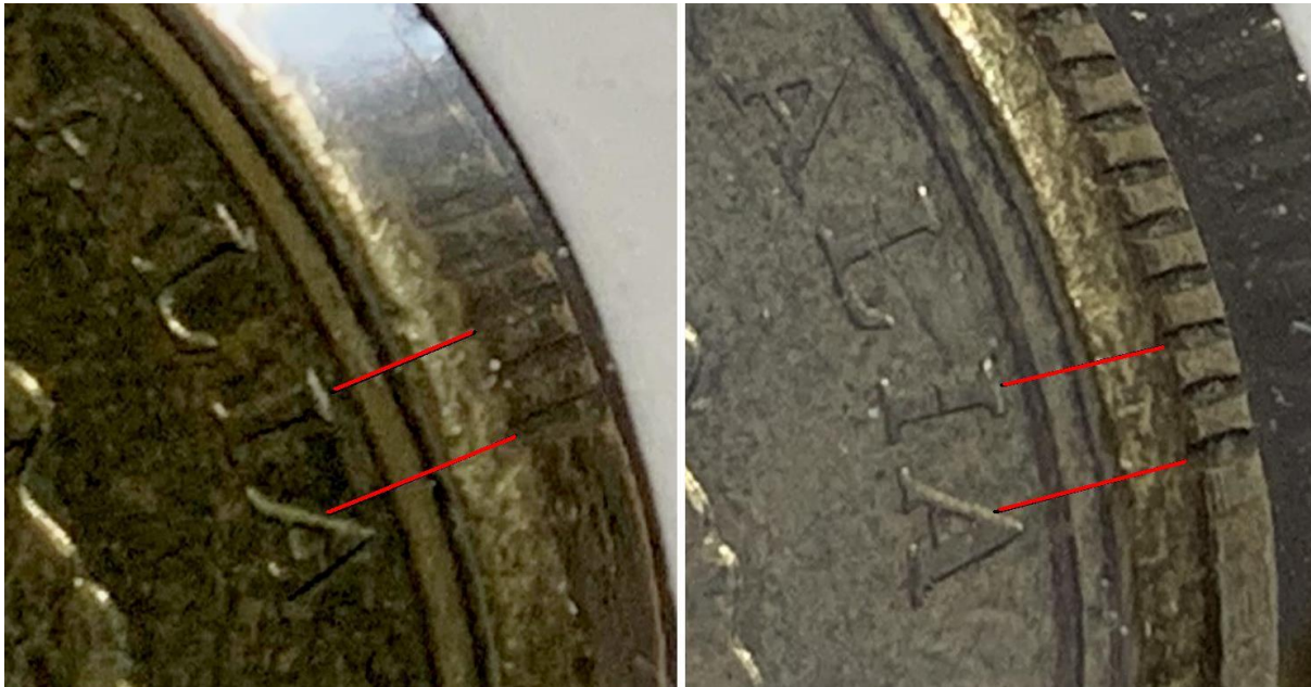
Fig 5. Alignment of the interrupted milling on two 2000 $1/10c mules. This is identical on all examples and is a firm indication that all coins were due to just one die pair.
