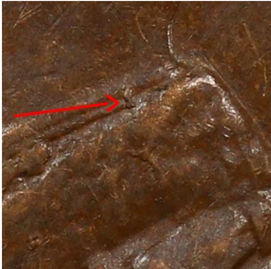
Fig 26. Tiny die flaw on HM's collar on the second die pair of the 1920 dot below, English obverse penny. Photograph courtesy of PCGS.
