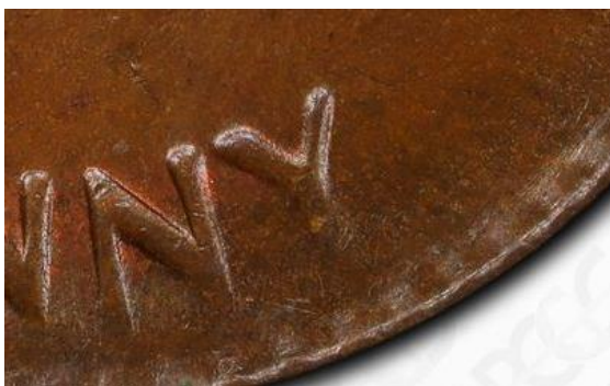
Fig 3. 1941 Penny with mintmark missing due to die fill. Photograph courtesy of PCGS.
