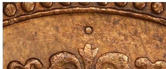
Fig 27. Dot below bottom scroll and dot above top scroll on a 1920 double dot penny. The dot below the scroll disappears due to die fill on later die state pennies. Photograph courtesy of PCGS.
