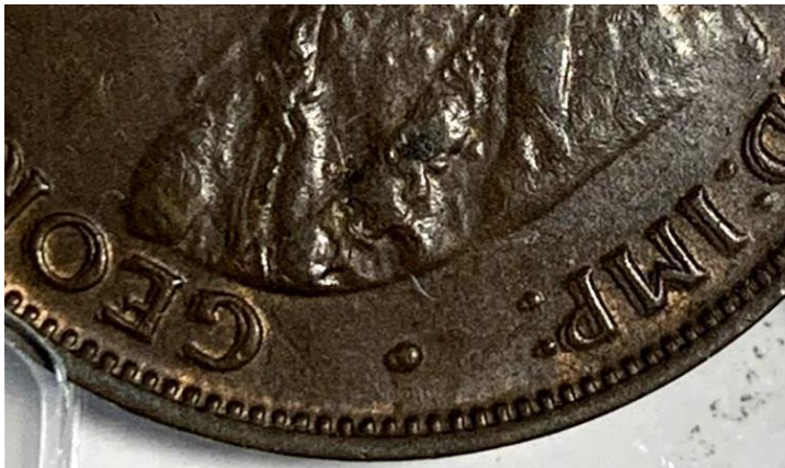
Figure 7. Hub doubling on a 1926 halfpenny. In this case the pivot point is on the rim at about 12 o'clock.
