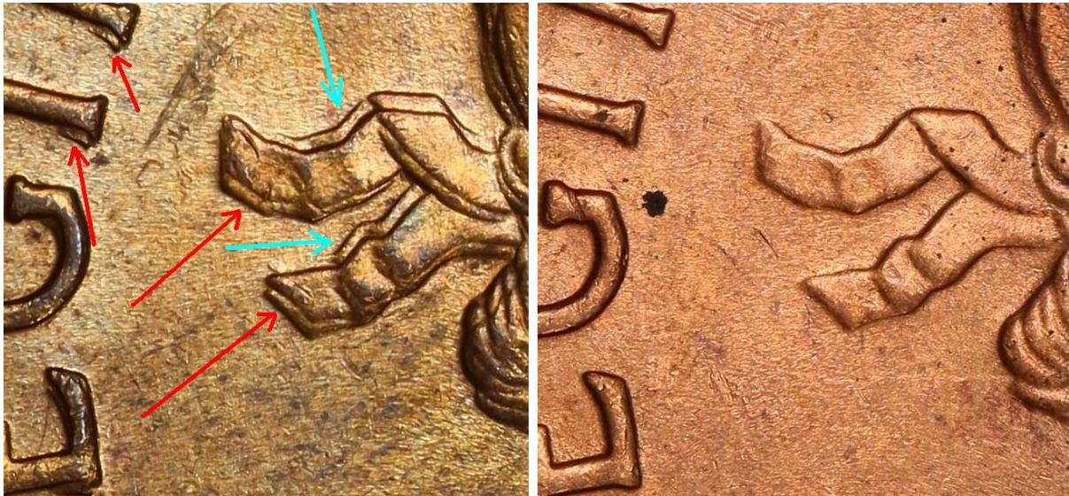
Figure 9. Comparison of double nose penny (left) with normal 1962 penny (right). Aqua arrows indicate features from first blow of the transfer punch, red from the second. Original photographs courtesy of PCGS.
