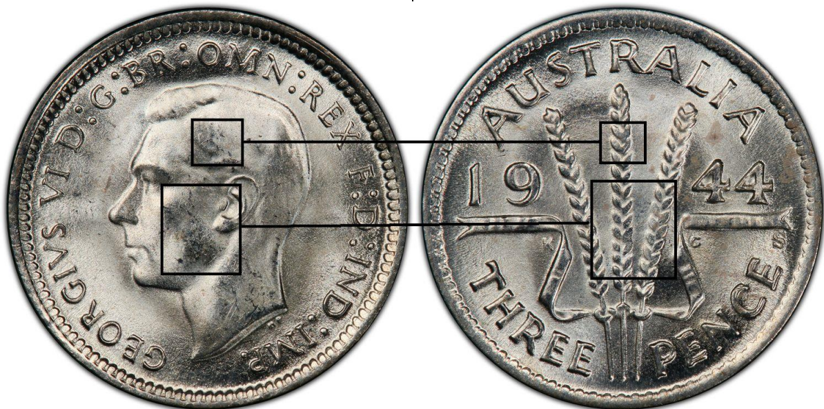
Fig 4 (part). Weakness on the reverse of a threepence as a result of high points on the obverse.
