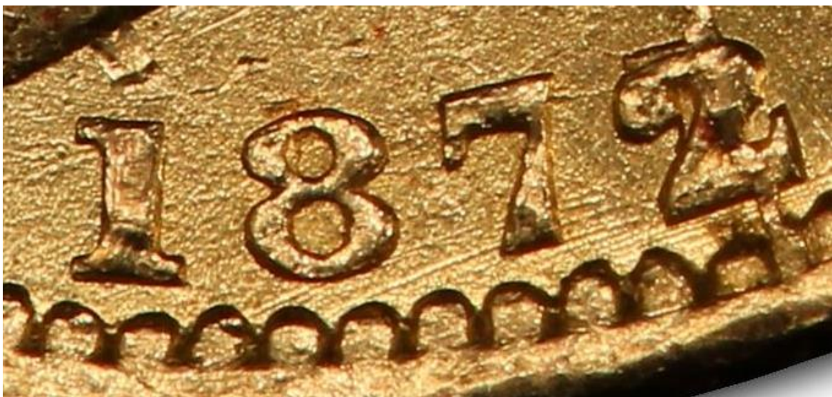
Figure 1. Close up of the date on an 1872/1 sovereign. Note the die crack that has developed through the 2. Engraving or stamping a digit over a pre-existing digit can cause die weakness. Photograph courtesy of PCGS.
