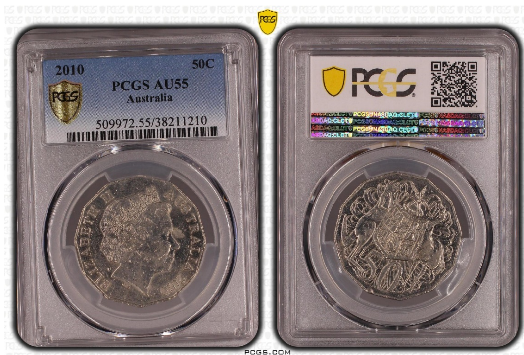
Figure 1. 2010 50c at 30 degrees rotation, an example of die misalignment. Photograph courtesy of PCGS.
