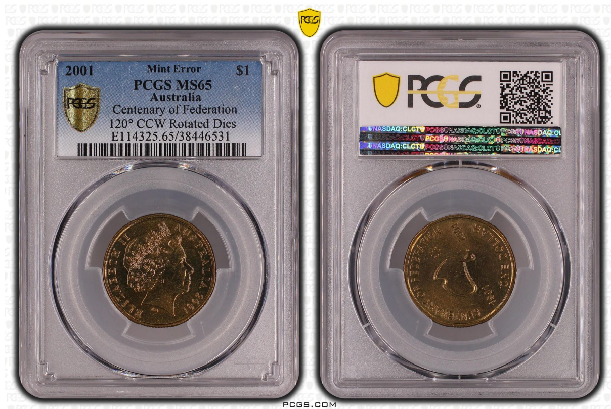
Figure 2. 2001 $1 Centenary of Federation rotated at 120 degrees, an example of machinery malfunction. Photograph courtesy of PCGS.
