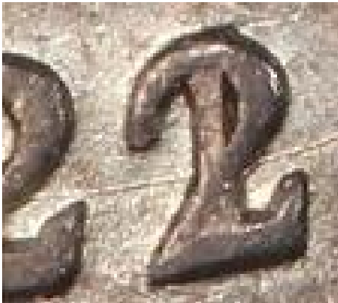
Figure 11. Closeup of the 2 on an overdate. Notice how the upper part of the 1 is thinner than the lower. This would have been caused by the metal forming the edge of the incuse 1 on the die being pushed aside by the 2 punch. Photograph courtesy of PCGS.
