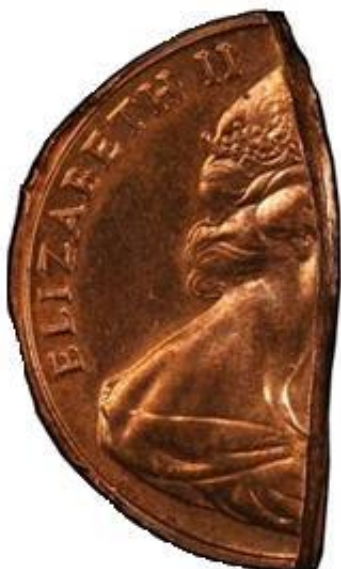
Figure 10. 2 cent, end of bar clip. Photograph courtesy of PCGS.
