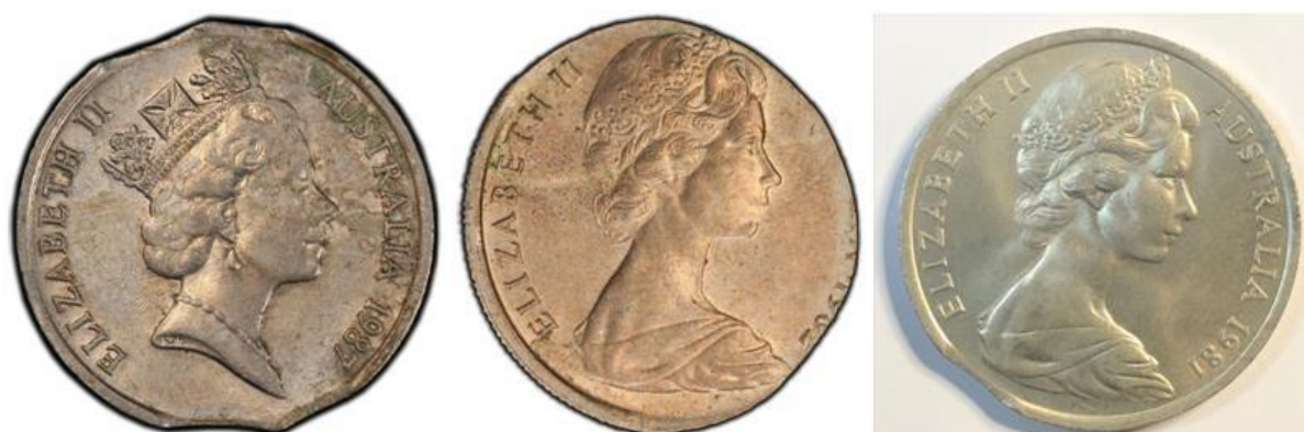
Figure 9. Quadruple clipped, elliptical and rim clipped planchets. The middle photograph is courtesy of PCGS.
