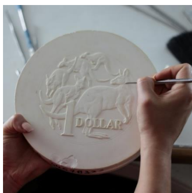
Figure 2. Plaster for reverse of $1 coin. Photograph courtesy of the Royal Australian Mint.
