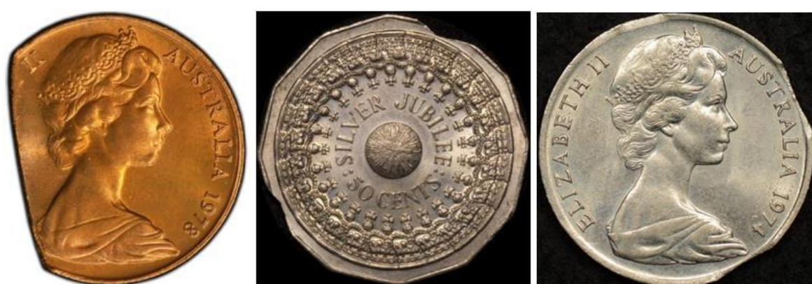
Figure 8. Ragged edge, double clipped and triple clipped planchets. Photographs courtesy of PCGS, Sterling & Currency, and the Purple Penny respectively.
