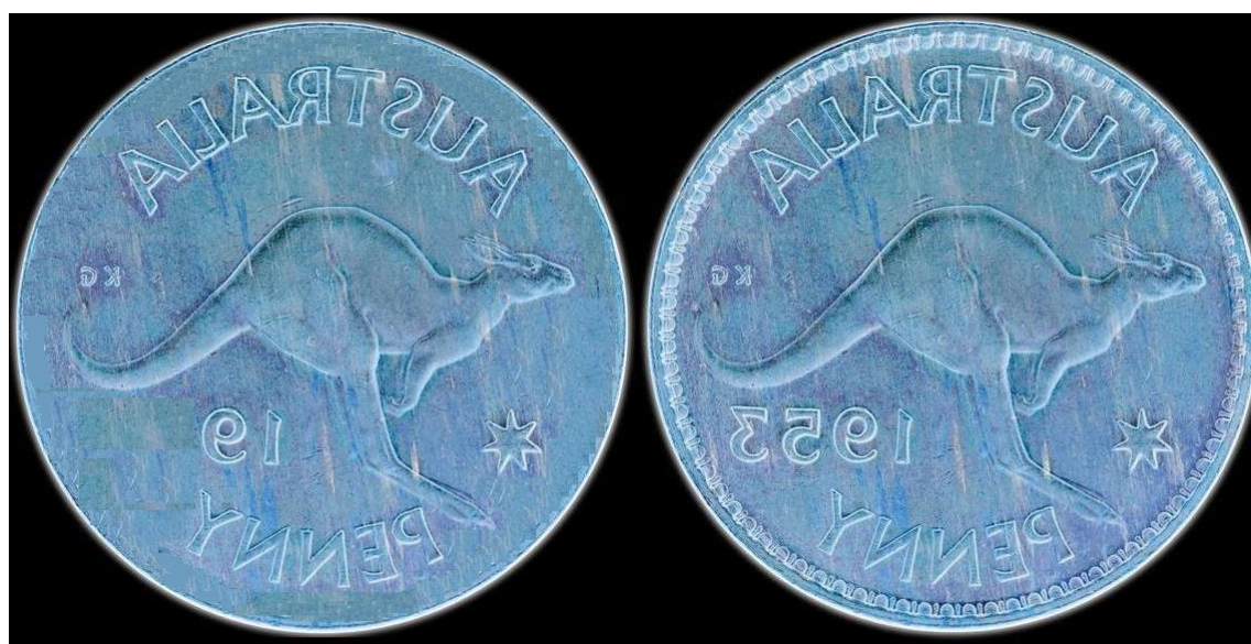
Figure 4. softened steel block (left), 1953 dated hub (right). Both have an incuse relief.
