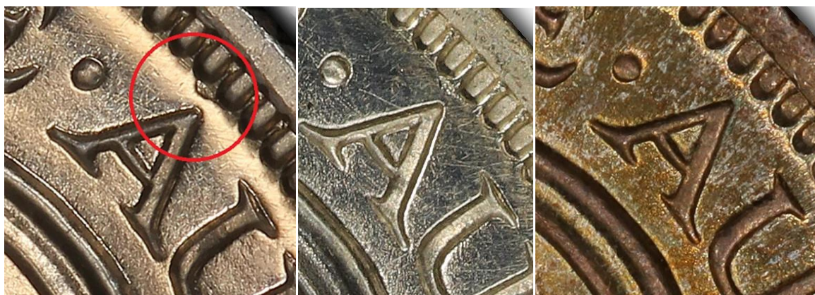
Figure 1. Chip above A – business strike using proof dies (left), proof coin (middle), normal business strike with no chip (right). The first photograph is courtesy of David Robinson, the other two courtesy of PCGS.
