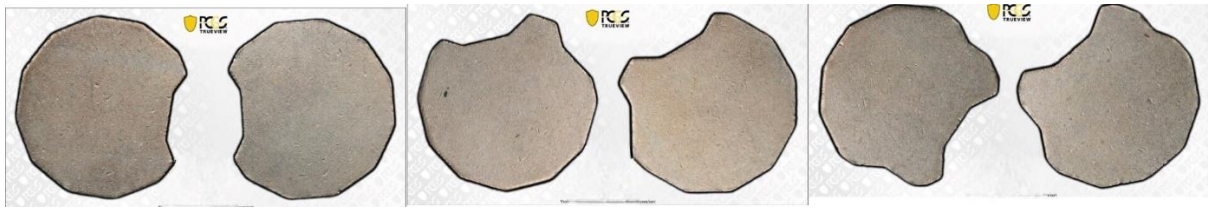
Figure 3. Typeset of clipped (single, double & triple) 50 cent blanks. Photograph courtesy of PCGS.
