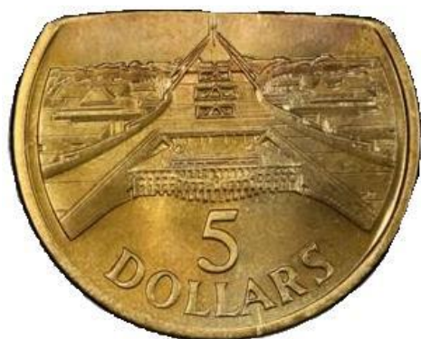
Figure 11. 1988 $5 40% straight end clip. Photograph courtesy of PCGS.
