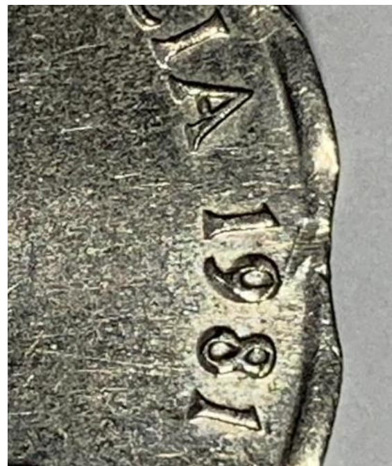
Fig 4. Indented lettering on the scalloped 20c due to unconstrained metal flow. Notice how this is more severe where the collar is not engaged such as the 9 in the date. Note also that the 'top' of the lettering is fully formed.
