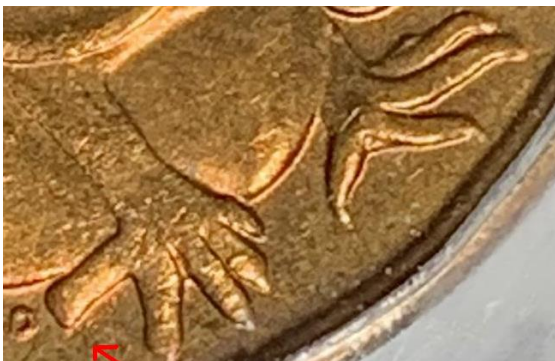
Fig 8. Perth Mint. Missing first claw on right foot.
