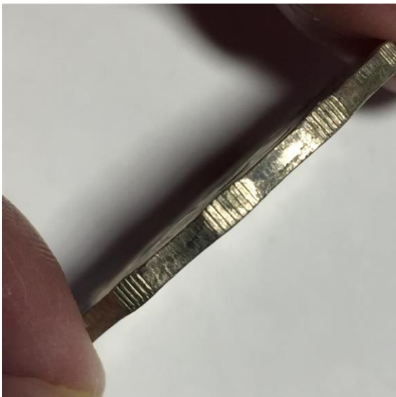
Fig 3. Edge of scalloped 20c showing engagement of the 20c collar.
