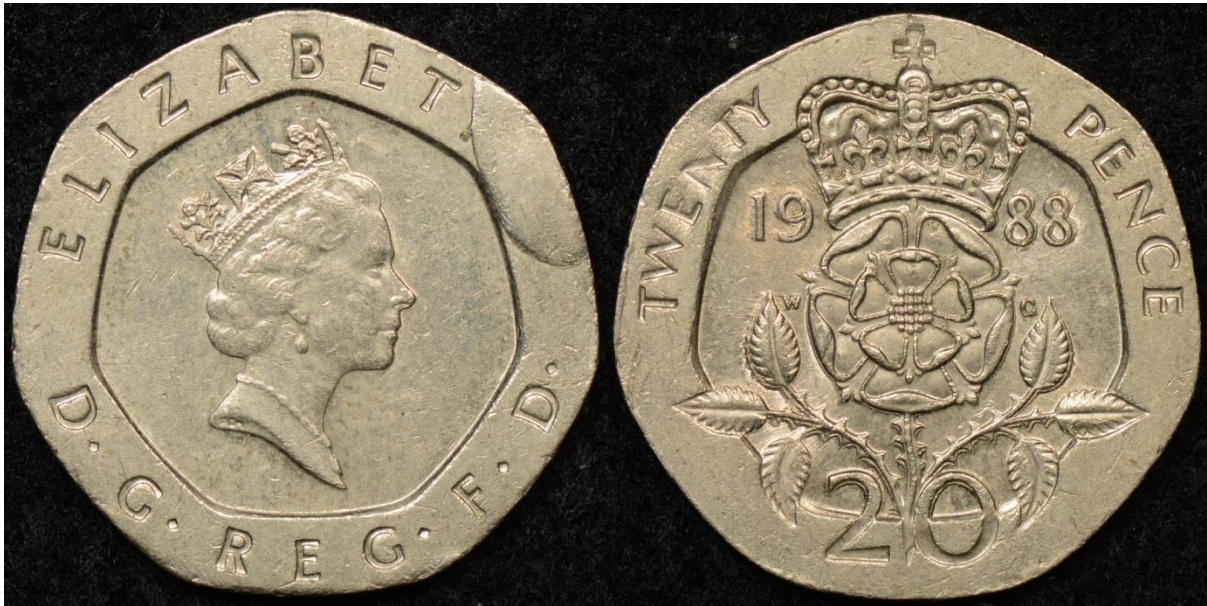
Figure 1. 1988 British 20p with a large obverse rim cud error. Image courtesy of the Purple Penny.
