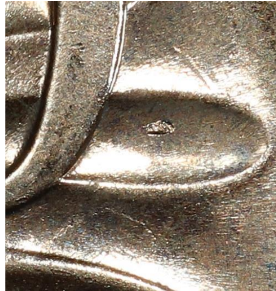
Fig 3. Die chip in swirl of Royal Mint coins. Original image courtesy of PCGS.
