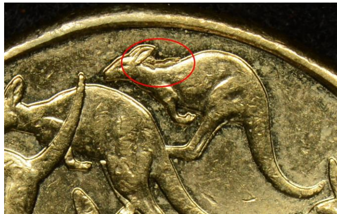
Fig 2. While often referred to as a rabbit ears cud, technically this is a die chip as the break in the die is not associated with the rim.
