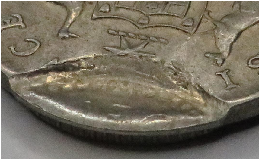
Figure 8. Indent on a sixpence. DEI of DEI GRATIA is visible at 12 o'clock on the reverse which is part of the legend normally only seen at 6 o'clock on the obverse. The previous coin had not quite cleared the press when this planchet entered and was struck over the edge of the previous coin. Indents are one off occurrences whereas partial brockages should create multiple error coins. Photograph courtesy of Gary Tate.
