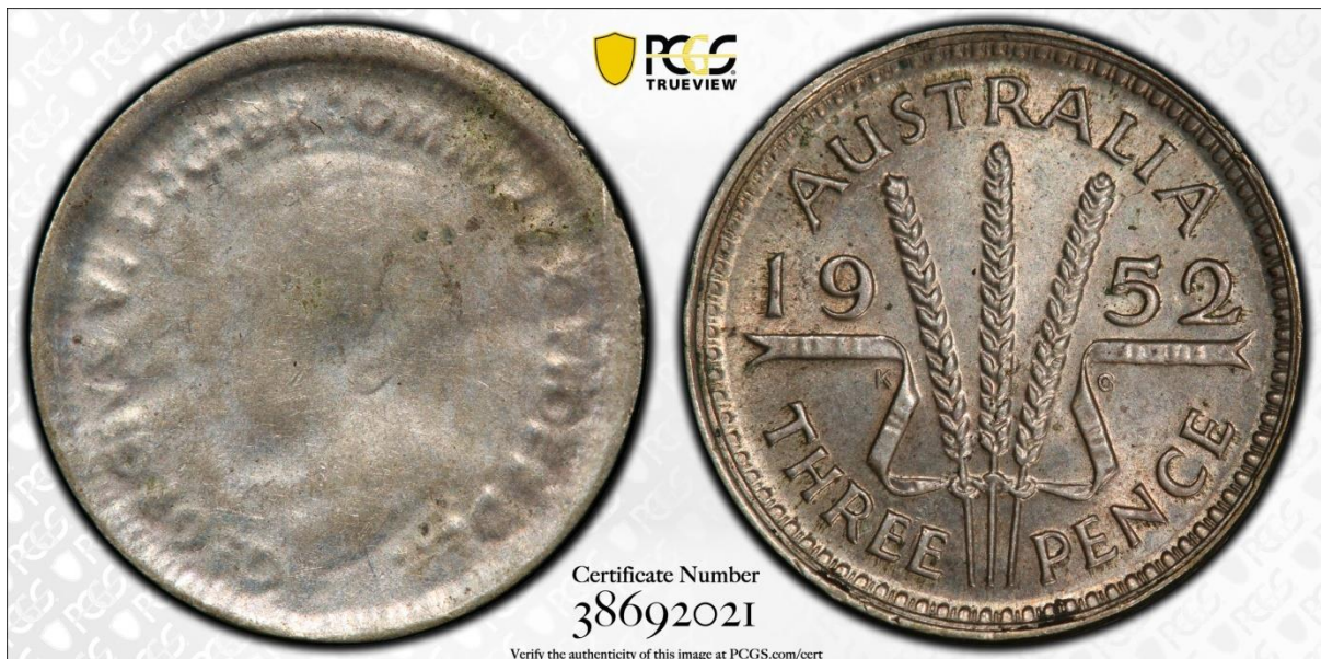
Figure 4. Struck through capped die error. Photograph courtesy of PCGS.
