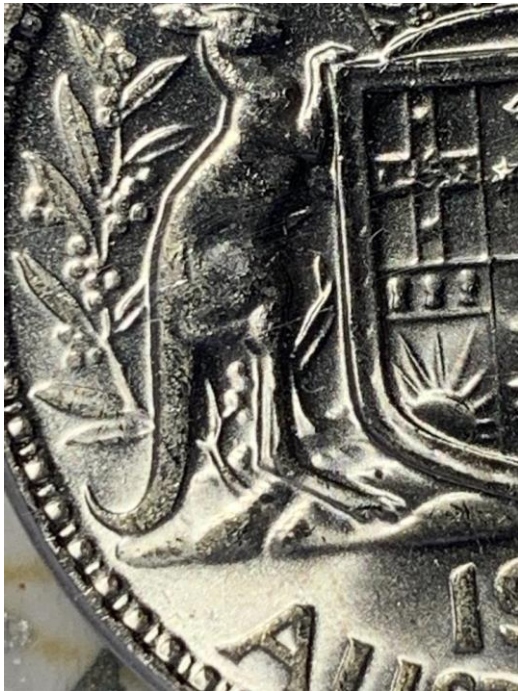
Figure 12. Roll rub on haunch of kangaroo due to coins rotating in a loose roll.
