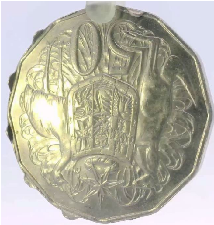
Figure 3. "Lugs" on ramstrike 50 cent at maximum. Photograph courtesy of Elliott Numismatics.
